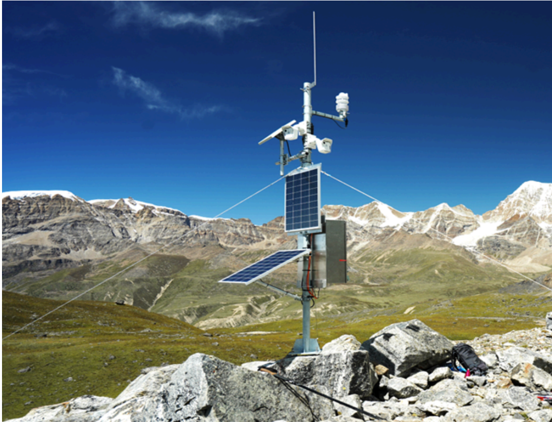
Figure 7: An AWS with webcams and lake water level monitors has already been installed at Shako Chho Lake. This independent data, along with field-level monitoring, will help provide a robust monitoring framework for the lake-level-lowering project.
