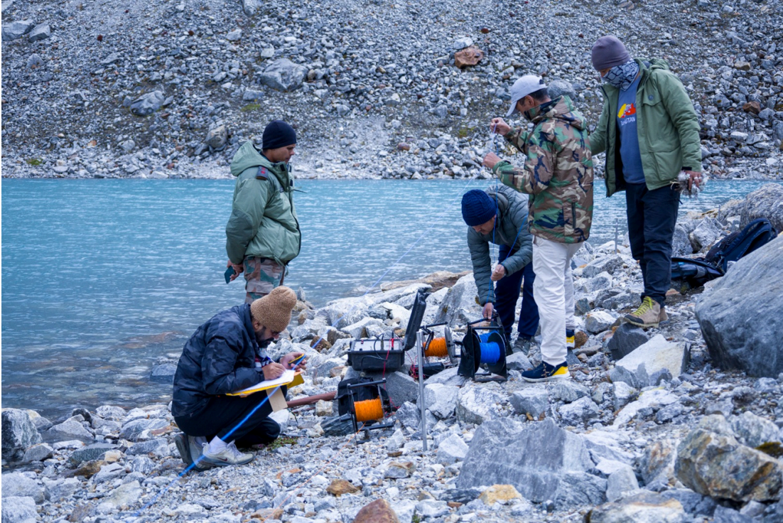
Figure 5: Geologists from the Department of Mines and Geology undertaking a subsurface geophysical assessment of the Shako Chho in 2024 to ascertain the stability of the terminal moraine
